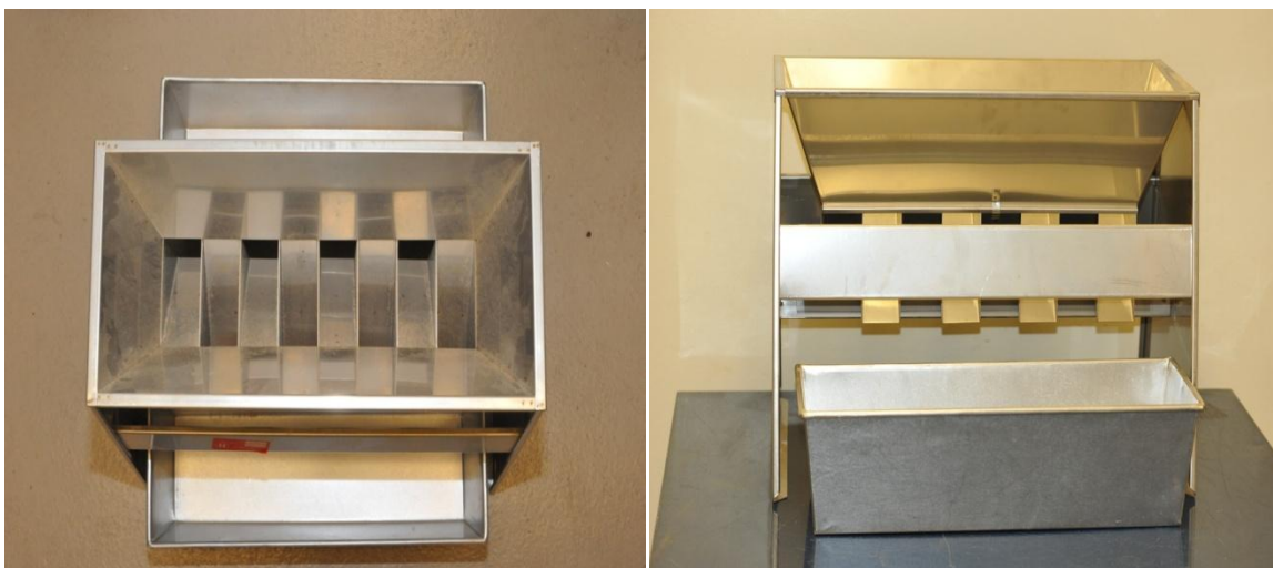
Figure 2.3 Hoffman R89P Riffle divider (Hoffman MFG, Jefferson, OR) used for randomly dividing a batch of pellets into two sub samples.
