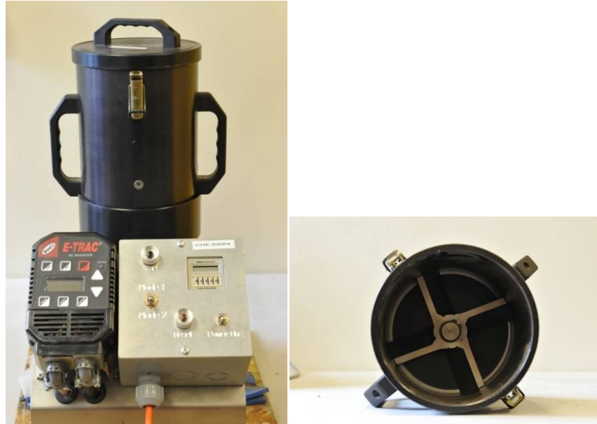
Figure 2.1 The picture on the left shows a Dural tester for durability measurement. The picture on the right shows the test housing and the rotating blades.
