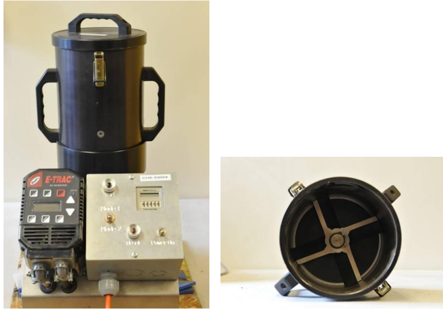
Figure 1.5 The picture on the left shows a Dural tester for durability measurement. The picture on the right shows the test housing and the rotating blades.
