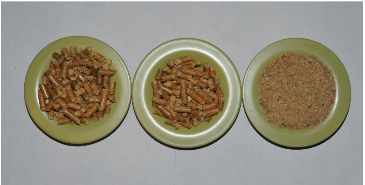
Figure 3.2 Surface breakage in pellets when impact forces are mild: original pellets (left), pellets after surface breakage (middle), and dust from surface breakage (right).
