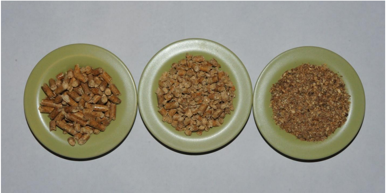
Figure 3.1 Volume breakage in pellets when impact forces are severe: original pellets (left), pellets after volume breakage (middle), and dust from volume breakage (right).
