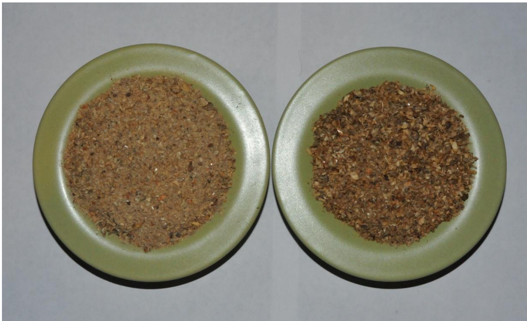
Figure 3.3 Side by side comparison of dust from surface breakage (left) and volume breakage (right).
