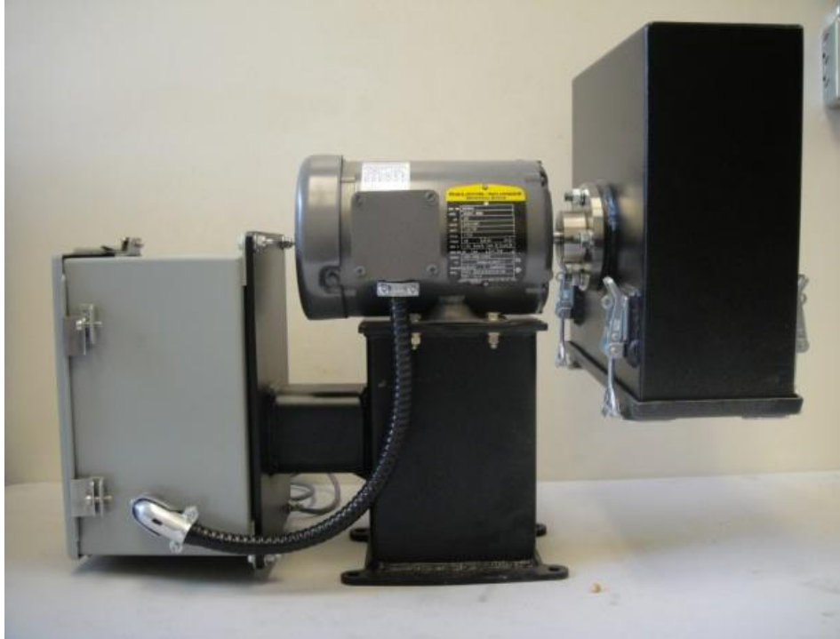
Figure 1.4 Tumbler tester for durability measurement
