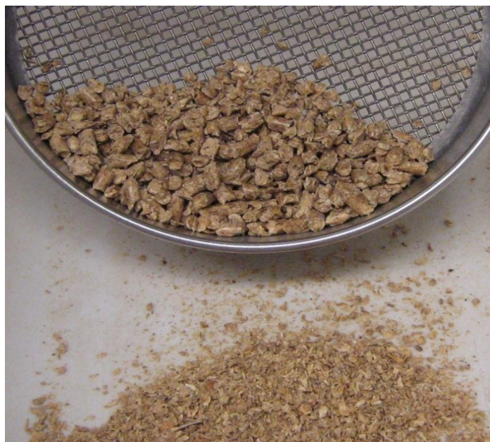
Figure 2.2 A 3.15 mm wire mesh screen used for removing fines and particles from pellets.
